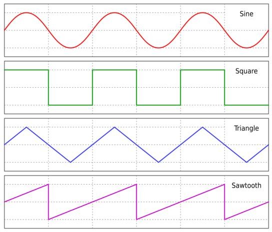
These signals are mixed together to produce a more complex waveform. Some of the signals can be used as modifiers to other oscillators, shifting the frequency based on a pattern.
